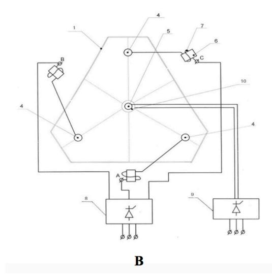
Figure 1. Slit (A) and cross cut (B) of electromagnetic technological reactor.
