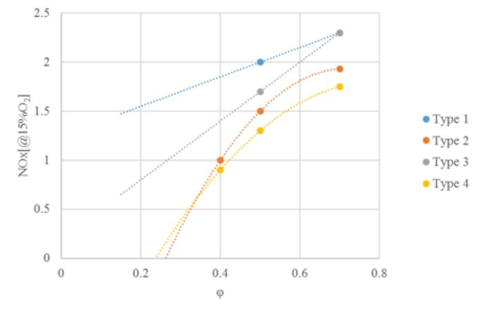
Figure 4. Dependence of NOx emissions on  $\phi$  and V-gutter type in variant 1 of fuel supply
