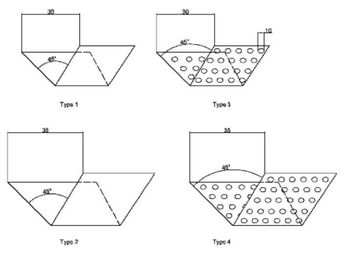
*Figure 2*. General view of V-gutter flameholders
