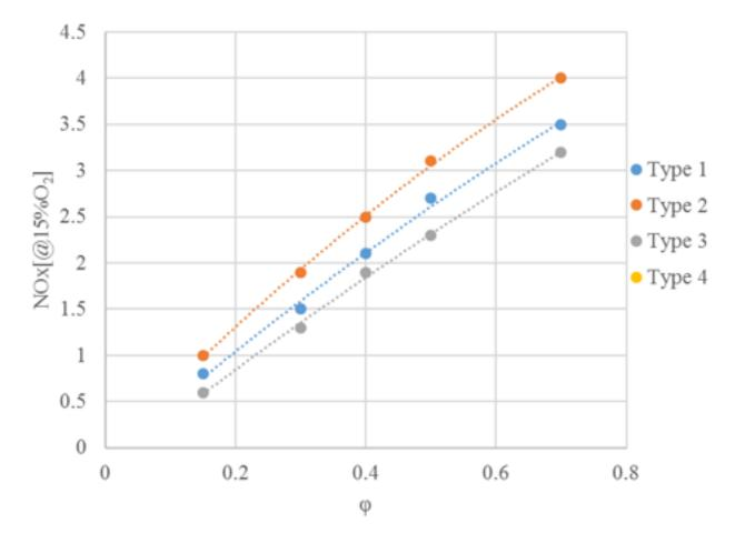
*Figure 5*. Dependence of NOx emissions on  $\varphi$  and V-gutter type in variant 2 of fuel supply
