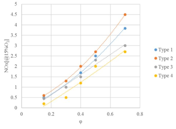
Figure 6. Dependence of NOx emissions on  $\phi$  and V-gutter type in variant 3 of fuel supply
