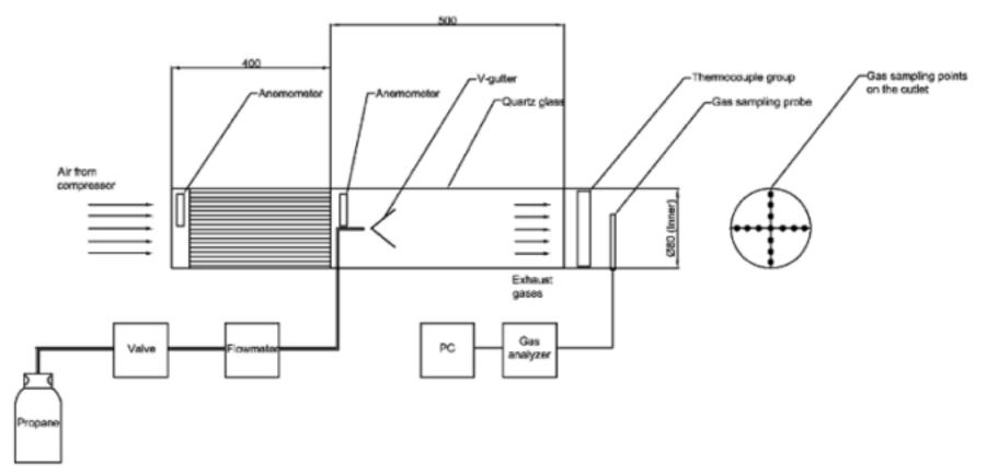
*Figure 1*. The schematic diagram of the experimental setup
